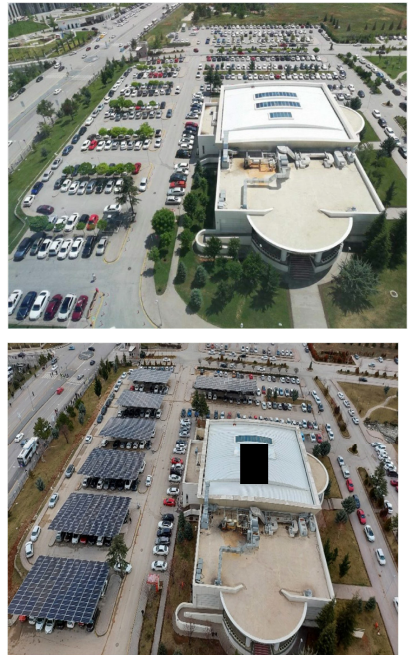
Picture 6. Parking lot carport solar photovoltaics (Before vs After)
