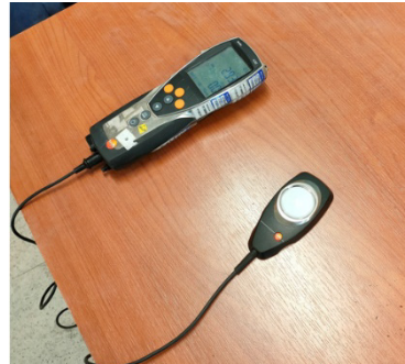
Picture 8. Illuminance level measurement
