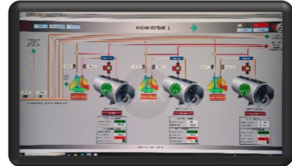
Picture 10. Building Automation and Energy Monitoring System
